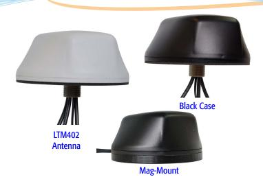
Mobile Mark's LTM402 Series Multiband Diversity/MIMO antenna contains four separate antennas, all in one compact antenna housing: two Global LTE/Cellular antennas, one 2.4/5 GHz dual-band WiFi antenna, and one GPS antenna. The LTM402 differes from the LTM401 in that it covers all LTE systems worldwide from 694-3700 MHz.
