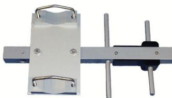
**YDM1 Dual Mount Kit:** YDM1 kit provides a second V bolt, and V block, and a mounting plate for greater boom support when used with larger Heavy Duty yagis that came with a single V bolt and V block assembly.
