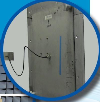
Swappable Antenna Horns from 450 MHz to 6.0 GHz shown on the outside wall
