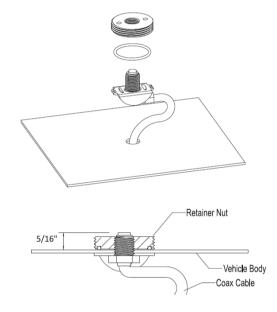
Drill a 3/8" (9.5mm) or 3/4" (19mm) hole in the car body at the desired location. Clean any burrs and paint from the area around the edge of the hole.
