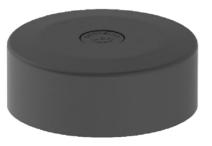
The antenna itself is totally self-contained and needs no tuning. The mounting pad allows for some variation in the flatness of the surface and provides a scratch resistant surface for mounting. The thickness of the mounting pad is critical to the performance of the antenna. It should be screwed on snuggly but not over tightened. It will withstand the effects of a car wash but it can be removed and reinstalled without any tools.
