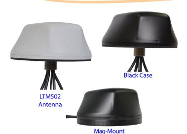
Mobile Mark's LTM502 Series Multiband Diversity/MIMO antenna contains five separate antennas, all in one compact antenna housing: two broadband LTE/Cellular antennas, two dual-band WiFi antennas, and one GPS antenna. The LTM502 differs from the LTM501 in that the broadband LTE/Cellular element covers all LTE frequencies worldwide, from 694-3700 MHz.
