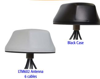
Mobile Mark's LTM602 Series Multiband Diversity/MIMO antenna contains six separate antennas, all in one compact antenna housing: two Global Cellular (up to 3.7 GHz) antennas, three dual-band WiFi antennas, and one GPS antenna.
