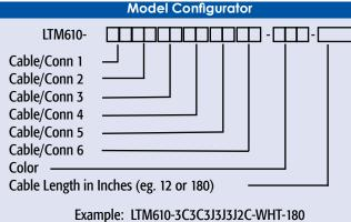
Specify "LTMG" instead of "LTM" for GPS/Glonass combination antenna.
