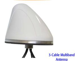
The SMW-310 Series Antenna has three separate RF cable feeds and will most typically be used for UHF, WiFi & GPS. Bandwidth coverage is 450-470 MHz on the first cable, 2400-2485 MHz & 4.9-6.0 GHz on the second cable and 1575 MHz for GPS on the third cable.
