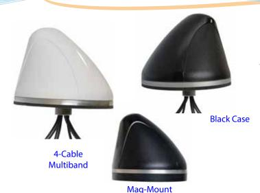
The SMW-413 Series Antennas features 4 elements in one antenna radome. The unique feature of this model is that the cellular element (Cable 1) is extremely widebanded and can cover: LTE at 700 MHz as well as the established 850/1900 GSM/CDMA bands, 1.7/2.1 GHz AWS and 2.5 GHz WiMAX all on a single board.
