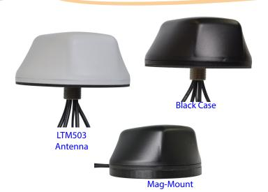
Mobile Mark's LTM507 Series Multiband Diversity/MIMO antenna contains five separate antennas, all in one compact antenna housing: two broadband LTE/Cellular antennas, one dual-band WiFi antenna, one Iridium antenna and one GPS antenna. The LTM507 differs from the LTM501 in that it covers the Iridium frequencies from 1616-1626.5 MHz.
