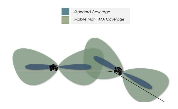
A Mobile Mark TMA has even greater reach than a 8dBi stick antenna, but it has the broader beam width of a 2dBi antenna, as illustrated below. The extra beam width allows the signal to reach higher and lower elevations to maintain connections at most angles encountered in a mine.
