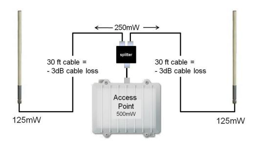
one per side (two total). As seen in the graphic above, the 500mW is reduced to approximately 125mW in a typical implementation, rendering it ineffective due to insufficient power to provide the needed
