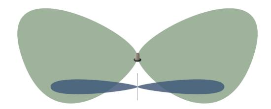
**Receive Gain.** Bi-Directional Signal Boosting: The Mobile Mark TMA incorporates a patented bidirectional Signal Boosting technology that cleanly amplifies the signal and further enhances the ability to maintain a strong connection with mobile clients on the network. In addition to delivering 20dB of transmit gain, 15dB of receive gain pulls the signal from low-powered client devices, delivering a more reliable and stable connection.
