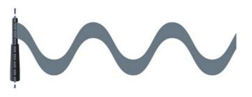
Figure 4: Example of Linear Polarized antenna misalignment
