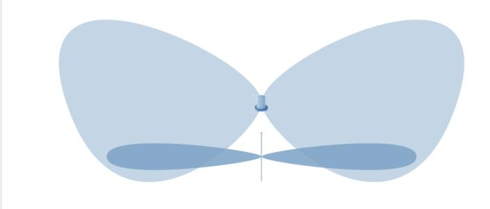
Figure 6: HP-TMA signal pattern compared to 9dBi Linear Omni signal pattern\*
