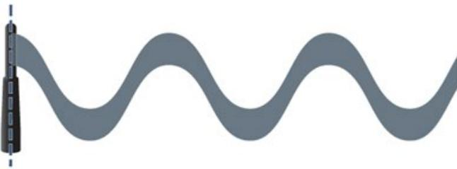
Figure 4: Example of Linear Polarized antenna misalignment
