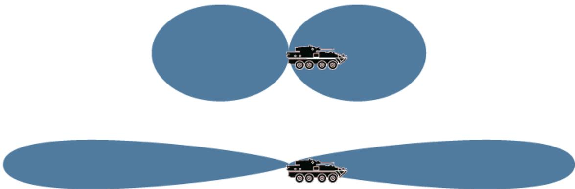
Figure 2: Representation of typical signal pattern of vehicles using 5dBi omni\*
