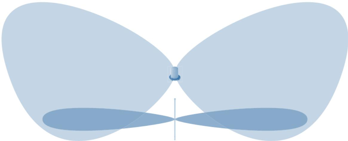
Figure 6: HP-TMA signal pattern compared to 9dBi Linear Omni signal pattern\*
