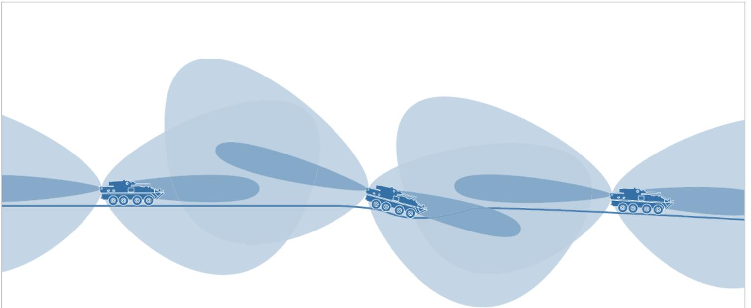
Figure 7: When vehicles pass over uneven surfaces, the broad signal pattern of the HP-TMA keeps vehicles connected, while the narrow signal pattern of a 9dBi Omni Linear Antenna allows connection to be lost\*
