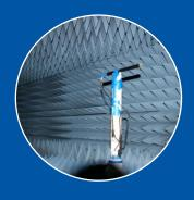
Anechoic Chamber for Antenna Characterization
